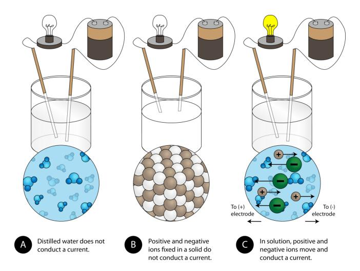
The tests of conductivity shown above are somewhat crude because a number of factors come into play when determining the resistance of a solution to conducting electricity. These factors include concentration of the solute, distance between the probes, and also how far into the solution the probes are placed.
