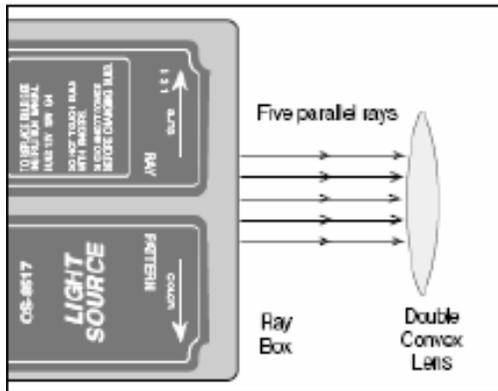
Note: Concave and Convex lenses have only one flat edge. Place flat edge on surface. Trace around the surface of the lens and trace the incident and transmitted rays. Indicate the incoming and the outgoing rays with arrows in the appropriate directions.
