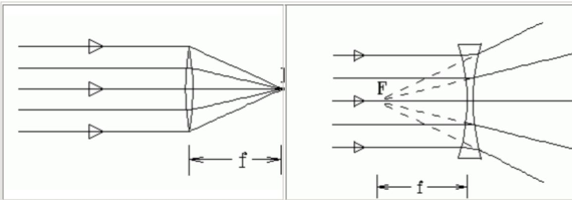
(c) A lens which **converges** a bundle of parallel rays is called a **converging lens**, or **positive lens** (its focal length is taken as positive). The converging lens is thicker at its center than at its edge.
