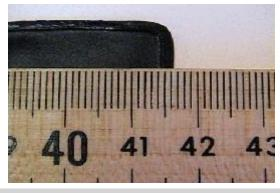
**Figure 2.** An example of a meter sticks reading. The object's length is measured to be 41.64 cm. (See text for description.)
