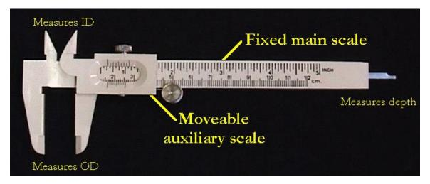
Their spacing is not the same as that of the marks on the main scale. If you look at these closely you will see that ten divisions of the Vernier scale occupy a length interval equal to *nine* of the smallest main scale divisions (millimeters). Obviously, in this case, the Vernier scale markings are engraved 9/10 millimeter apart.
