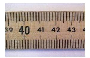
**Figure 1.** This meter stick is calibrated in centimeters (shown as the numbered major divisions) with a least count of millimeters.
