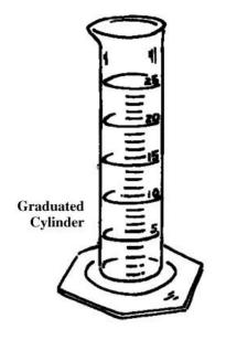
The instructor will explain how to read a graduated cylinder, especially what is meant by the "meniscus" and how to avoid the error of *parallax* in reading the level.
