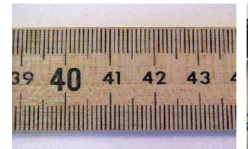
**Figure 1.** This meter stick is calibrated in centimeters (shown as the numbered major divisions) with a smallest number of millimeters.
