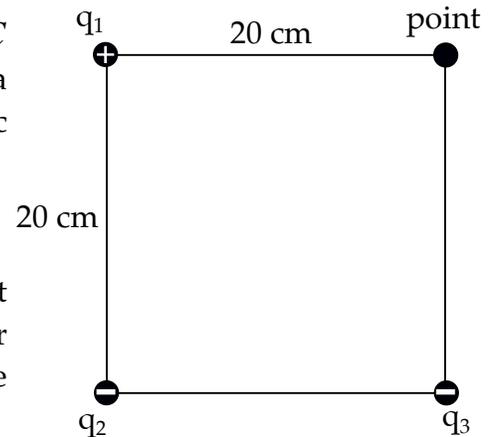
Solution 1: since electric potential is a scalar, the net potential is a simple algebraic sum. (No vector addition.) Remember,  $q_2$  is across the diagonal of the square to the point, so  $r_2 \approx 28.3 \text{ cm}$ :
