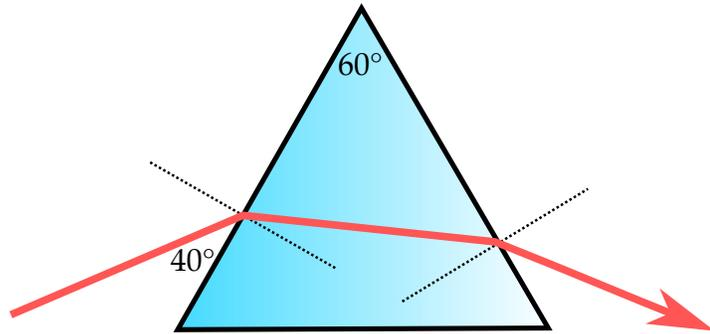
Solution: this is a two part problem: air-to-glass refraction as the beam enters the prism, and glass-to-air as the beam exits the prism.
