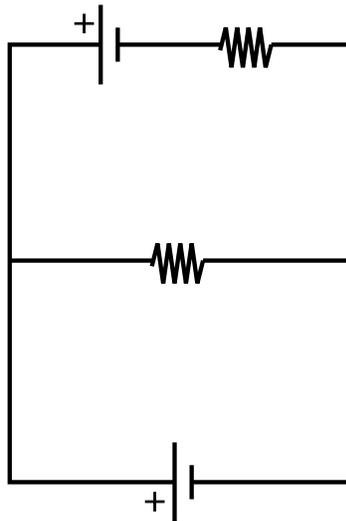
Three-branched circuits have three branches joining the two junction points. They also have three loops, which I call the top loop, the bottom loop and the outside loop.
