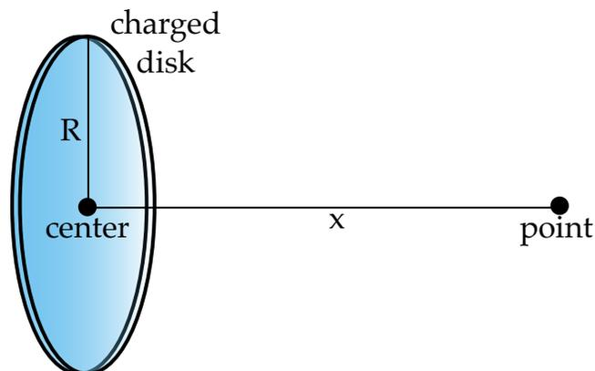
Solution: a disk can be thought of as an infinite series of rings (circles) with increasing radius. The strategy is to begin with a circle of charge of radius  $y$ , and infinitesimal width  $dy$ , and take an infinite summation (integrate) from 0 to  $R$ .
