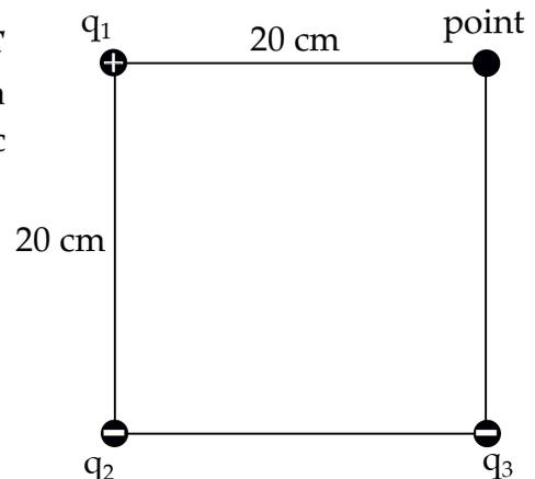
Solution: since electric field is a vector, you need a vector diagram with the point at the origin. Notice,  $q_2$  is across the diagonal of the square to the point, so  $r_2 \approx 28.3 \text{ cm}$ .
