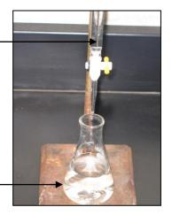
The picture above shows a titration apparatus. The experiment makes use of a buret that contains the sodium hydroxide solution. An Erlenmeyer flask contains the vinegar solution and a couple of drops of the indicator (phenolphthalein). The sodium hydroxide solution is poured into the vinegar solution one drop at a time. The volume of sodium hydroxide required to react with all of the acetic acid in the vinegar is measured from the buret.
